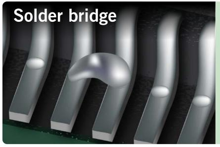
A solder bridge is a mechanical bridge formed by solder alloy between two component terminals resulting in an electrical short and circuit malfunction. In the reflow soldering process, solder bridges are mostly seen on fine pitch ICs. But in the wave soldering process solder bridges can be seen between terminals on a variety of components with larger pitch or between terminals of two chip components.
