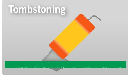
Tombstoning is a term in the chip soldering industry describing a situation wherein a soldering defect causes a chip component to stand up on end (like a tombstone), leaving one end soldered to the board and the other end free. It is caused during the reflow soldering process where non-uniform melting causes an unbalanced force to be applied to the chip from the solder.
